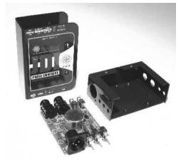
even the most gruesome noises, a ground lift is provided to isolate input and output grounds from the shell. Normally, when interfacing guitars and basses, lifting the ground (depressing the switch) should not be necessary. Sometimes, when using devices that are AC powered such as keyboards or amplifiers one will encounter additional noise. Trying the ground-lift may sometimes help.
