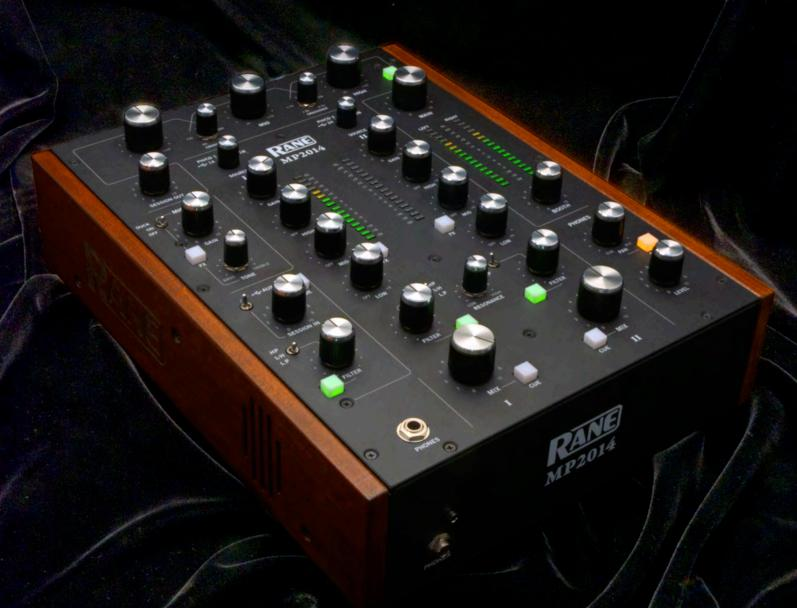
The MP2014 represents the perfect marriage of a high-quality rotary control-surface, with state-of-the-art digital signal processing and dual 16-channel USB sound cards. An essential assortment of analog and digital I/O supports mixing vinyl, CDs and USB streaming audio in any combination. Simple, elegant and easy to master.
