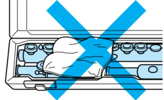
When closing the case, make sure there are no objects such as a gauze or cloth on top of the instrument. Doing so may put unnecessary pressure on the keys causing damage. Also, never leave a damp cloth or gauze, etc., in the case.
