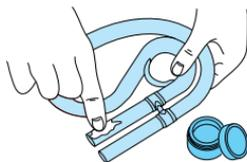
4. Slide the valve slide in and out a few times to distribute the grease evenly. Then wipe off any extra grease that comes off the slide.
