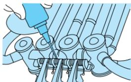
\* Remove excess oil and use a gauze cloth to clean the smaller parts.
