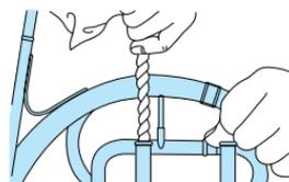
3. Use the gauze to remove dirt from the surface of the valve slide, then apply a little slide grease.
