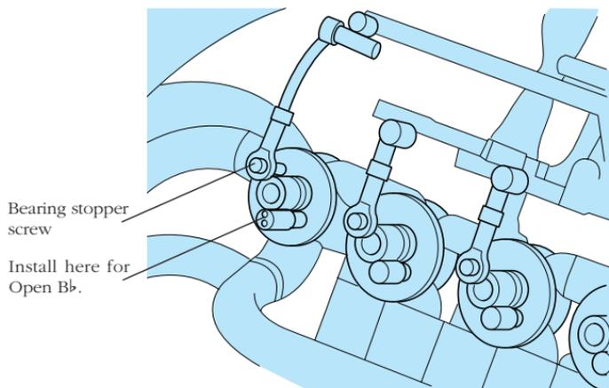
\* When the bearing stopper screw is installed near the rotating center, the stroke will become short. When the screw is installed far from the rotating center, the stroke will become long.
