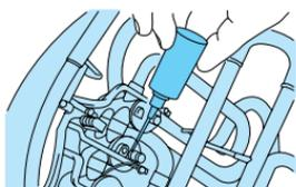
3. Apply a little lever oil to each linkage of the lever assembly.
