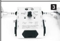
Connect cable: insert the testing cable into corresponding holes.
