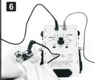
The application of probe line: insert two probe lines into banana jacks, if you hear buzzing and yellow LED light on, it indicates that the line is well. According to this method, to test audio cable which the inserting holes are not matching. Use probe pen to connect audio cable, if you hear buzzing it indicates that the line is well.
