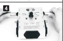
Test cable (one): twist the knob to the position of "1", if green and yellow light on at the same time, it indicates that PIN-1 of this line is well.
