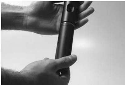
Figure 3 - Unscrewing M3 body
