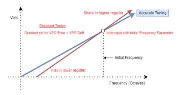
The above graph applies to FVPO Error, FVPO Drift, FDrift Speed and FInitFreq in relation to the filter where frequency is in relation to the frequency of the resonant peak of the filter; OSCVPO Error, OSCVPO Drift, ODrift Speed and OSCInitFreq where frequency is in relation to the pitch of the oscillators. These parameters allow the tuning of the filter to be adjusted emulating volts per octave calibration tuning error in vintage synthesizers.
