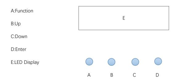
Instructions:Press the function key A cycled out the eight different function effects, digital tube first two digits on behalf of which the current function (see menu). The last two digits represent the functions in which the address code or speed parameters. Press the B or C key to modify the parameter values. Press the D key to confirm.
