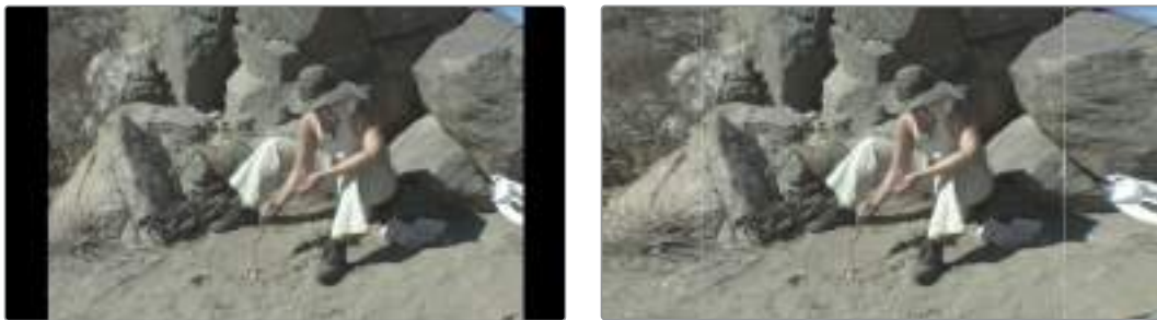
(Left) The original 4:3 image edited into a 16:9 timeline with black pillar boxing to the left and right as a result, (Right) The image with Blanking Fill set to Warp Top Layer, stretching the left and right edges to fill the blanking area
