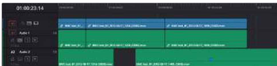
Deleting Clip I using the Forward Delete key to ripple all clips with In points to the right in the Timeline to close the gap
