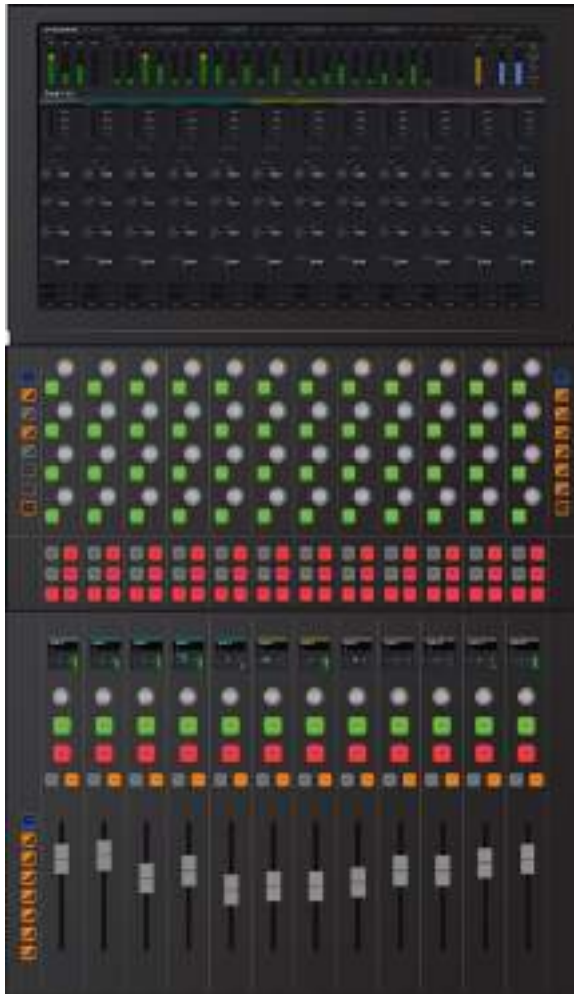
Channel Control components set to In-Line mode
