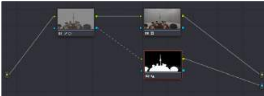
Connecting a key output to an RGB input to adjust a key used to create transparency via the Alpha output
