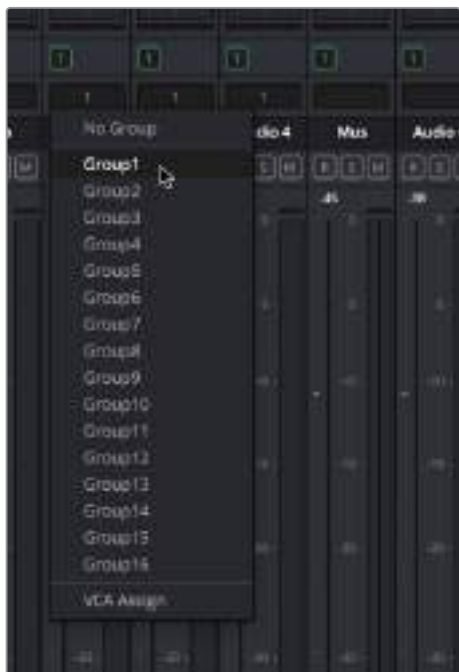
Right-clicking a Group Label reveals a drop-down menu that lets you assign faders to or remove faders from groups
