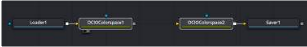
An OCIO Color Space node applied to a Loader node and a Saver node in Fusion Studio
