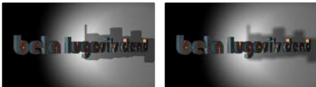
When the Renderer3D node " Renderer Type " pop-up is set to OpenGL Renderer , you cannot render soft shadows or excessively large textures (left). When the Renderer3D node " Renderer Type " pop-up is set to Software Renderer , you can render higher-quality textures and soft shadows (right).
