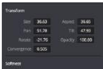
The Convergence control in the Transform section of the Window palette appears when you enable “Apply stereoscopic convergence to windows and effects”
