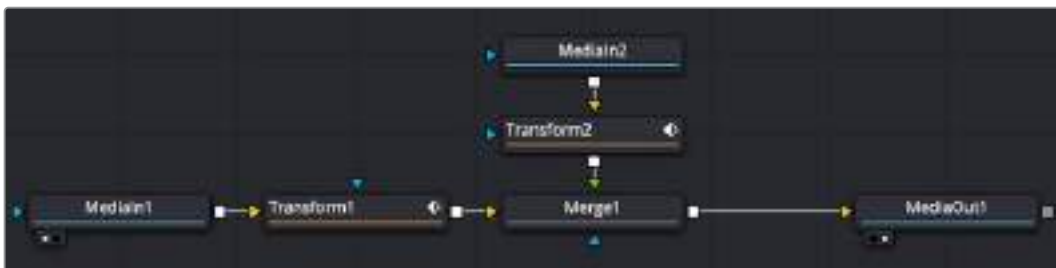
The Fusion Cross Dissolve node tree replaced with Transforms and a Merge node.
