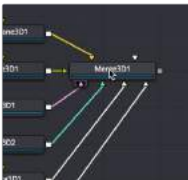
Hovering the pointer over a node highlights the color of all connections, telling you what kinds of inputs are connected.
