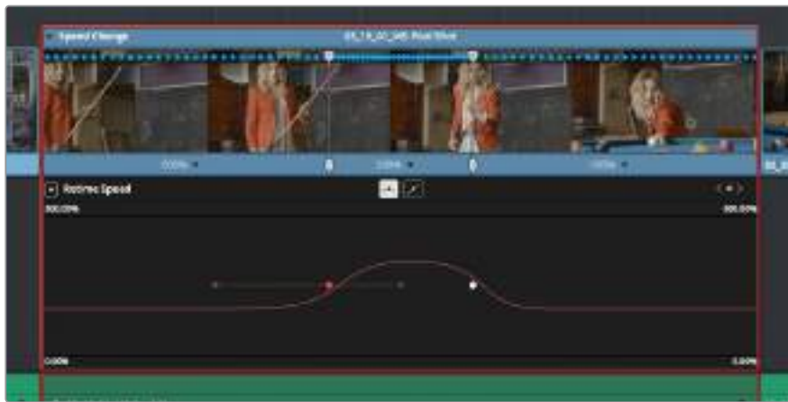
The Retime Curves let you adjust the transition from one speed to another using handles
