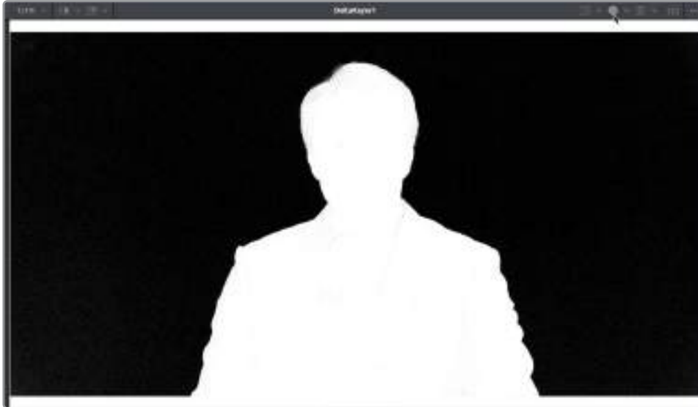
Loading the DeltaKeyer into the viewer and clicking the Color button to view the alpha channel being produced.
