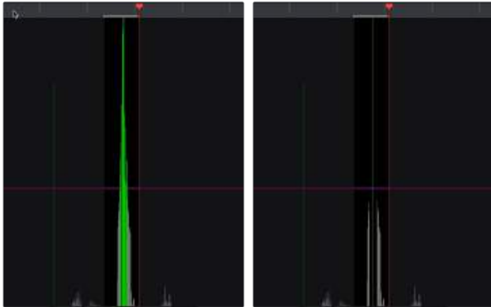
(Left) Isolating scene cuts to prune with In and Out points, (Right) The result of clicking the Prune button to eliminate all unwanted scene cuts but one
