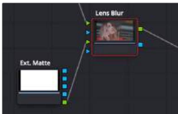
A Lens Blur node set up using a second RGB input with External Input Shape Type
