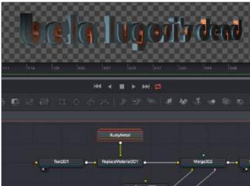
The geometry created by a Text3D node is textured using a shader connected to a ReplaceMaterial3D node that's connected downstream of the object you want to shade.
