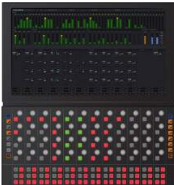
Channel Control components in Master mode
