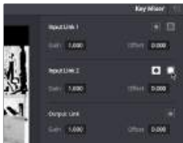
Turning on Matte and Invert for Input Link 2 to Output Node 3 subtracted from Node 2
